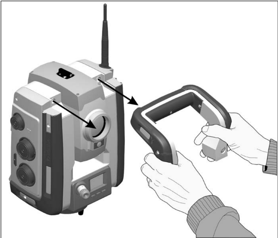
Figure 3.21 Detaching the instrument handle
