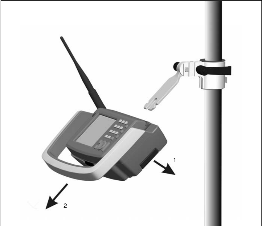
Figure 7.76 Detach Trimble Robotic Holder from stake writer rod adapter
