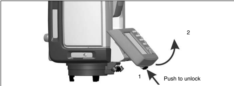
Figure 4.37 Detaching the Trimble CU
