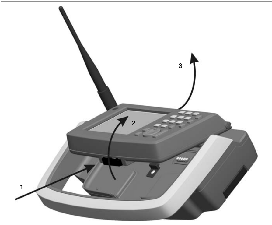
Figure 7.74 Detach Trimble CU from Trimble Robotic Holder
