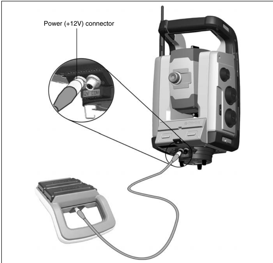
Figure 3.14 Connecting the Multi battery Adapter
