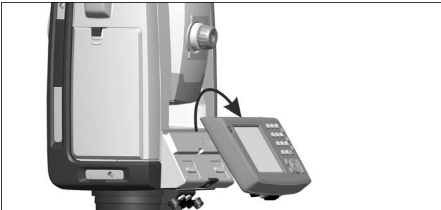
Figure 4.38 Detaching the Trimble CU
