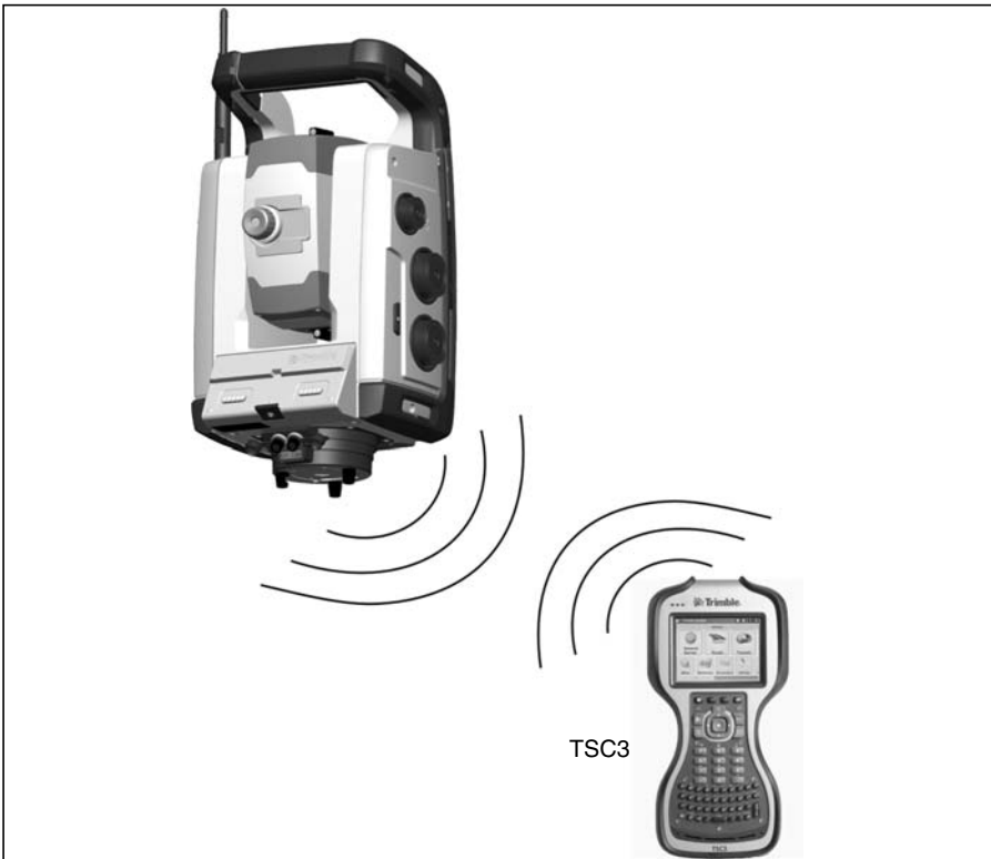
Figure 4.40 TSC3 connected to the Trimble SPSx30 Total Station with Bluetooth wireless technology for servo and Autolock measurements.
