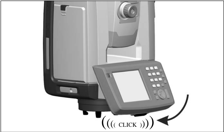
Figure 4.36 Attaching the Trimble CU
